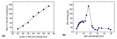
Fig. 2. Idler I<sub>2</sub> energy of the AGSe SRO at 11.46  $\mu$ m (normal incidence,  $\theta$ =51.3°) vs. pump P<sub>1</sub> energy at 1.064  $\mu$ m (a), and angle tuning of the AGSe SRO in the mid-IR at a pump energy of 55 mJ at 1.064  $\mu$ m (b).
